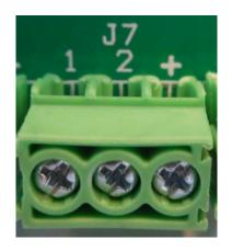
There are two open connector outputs, which can drive external relays, activate inputs in a control system, etc.
