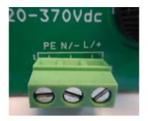
The power must be connected to the mains screw terminal (J1) as shown below.
