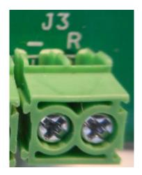
The counter may be reset via a push button or a relay contact connected to the two terminals labelled "R" and "-" in the connector J3.
