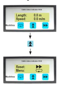
By pressing the "Arrow Up", you can either enter the menu or reset the cable counter as shown on the picture.
