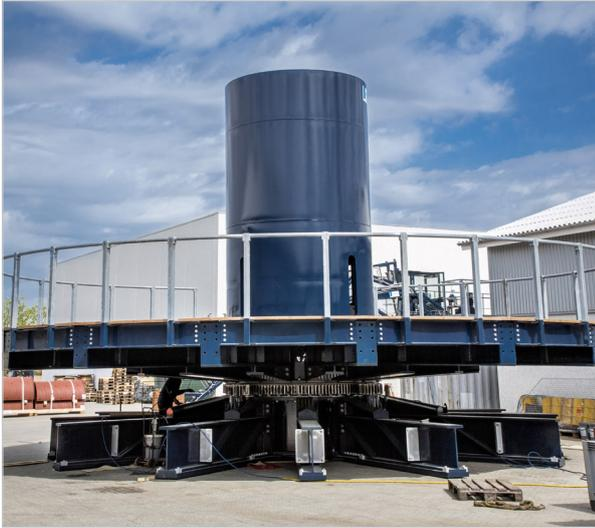
MacArtney's electrically driven CEMAC carousel solutions are robust and energy-efficient cable handling systems that safely store and install on- and offshore power and telecom cables.
